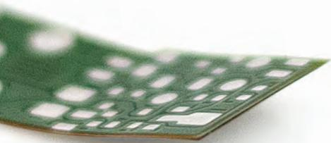
It's becoming more common to use laser depaneling, thanks to the benefits that this technology can offer in terms of cycle time, quality of the cut edges, dimensional accuracy of the cutting and the high flexibility that a laser cut can offer.
