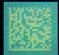
CO 2 color change on solder resist
