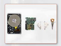
Recovering Rare Earths from the **Permanent Magnets** contained in end-of-life hard disks.
