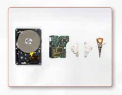
Recovering Rare Earths from the **Permanent Magnets** contained in end-of-life hard disks.
