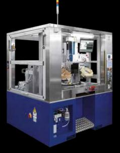
Single block basement with welded steel frame and integrated electrical panel. Operators can **easily** access the stations for maintenance purposes.
