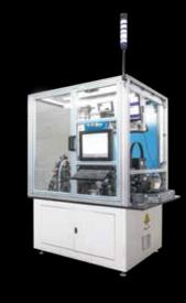
According to the connection diagram of the module, the system, guided by a vision system, will place the bus bars to be welded above the contacts of the cells and will check their position, preparing them for
