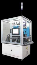
The system is capable of dispensing the glue and the heat conducting paste among the cells. The optical control and UV curing are integrated.
